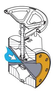
Series 2000 Pinch Valves provide excellent flow control compared to other valves due to their simple yet effective design. In addition, the sleeve is the only part of the valve exposed to the line process, eliminating corrosion of the more expensive mechanical components.
