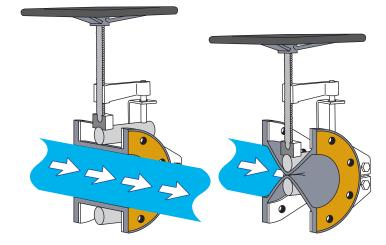
Series 1000 Pinch Valves provide excellent flow control compared to other valves, due to their simple yet effective design.
