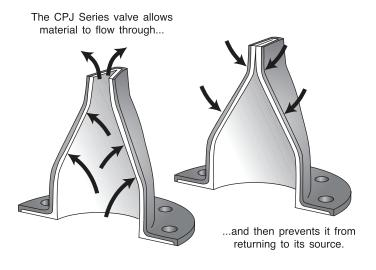
The heart of the Elasto-Valve Series CPJ Backflow Preventer is a fabric reinforced rubber "duckbill" sleeve manufactured with top quality materials. This flexible sleeve provides maximum flow with a minimum pressure drop across the valve at all times.
