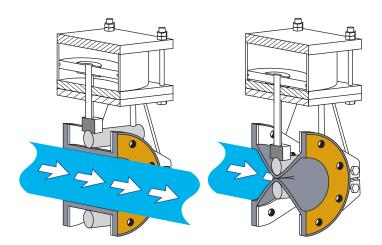
Series 1200 Pinch Valves provide excellent flow control compared to other valves due to their simple yet effective design.
