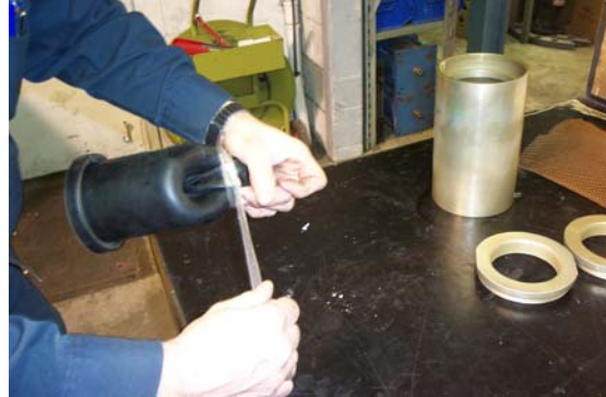
Picture 4 – Use tape to keep flange compressed (if required)
