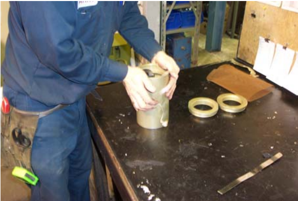
Picture 7 – Snap sleeve flange over valve seat
