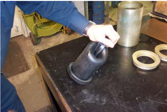
Picture 3 – Completely compress flange
