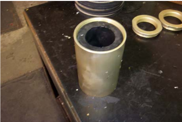
Picture 9 – Lubricate sleeve flanges prior to tightening end caps
