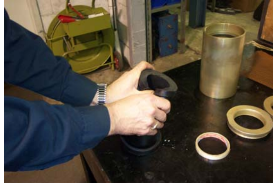
Picture 2 – Begin compressing one sleeve flange
