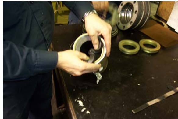
Picture 8 – Ensure sleeve flange is properly seated
