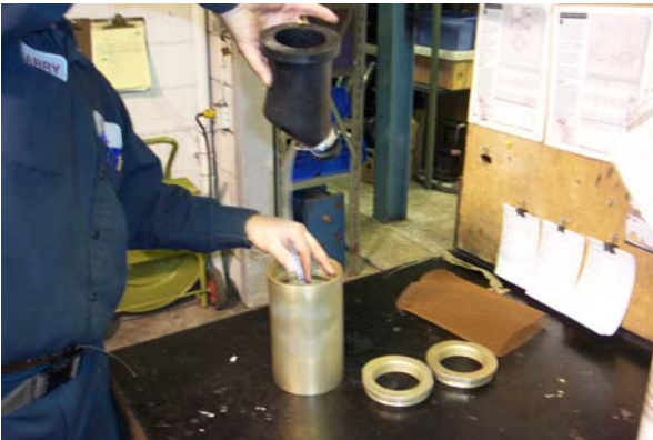
Picture 5 – Insert compressed sleeve flange into valve body
